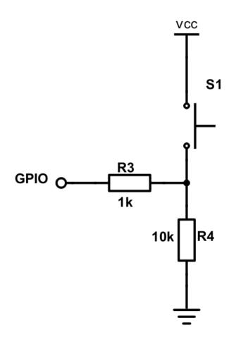
Figure 2. Button Switch Circuit Schematic
