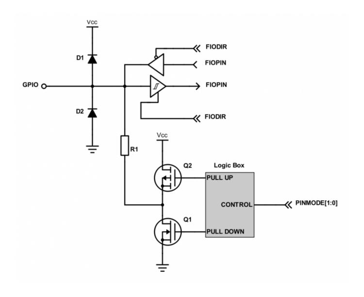
Figure 1. Internal Design of a GPIO
