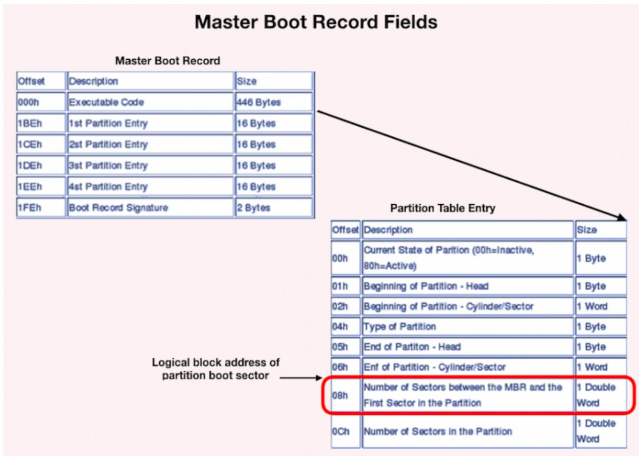
The first 446 bytes is the bootstrap code area. After that there is a partition table with four entries and then a boot signature (0x55AA). Each entry is 16 bytes long. To see the structure of the [Master Boot Record: Sector layout](#) and the structure of the entry can be found here [Master Boot Record: Partition table entries](#).
