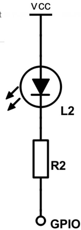
Figure 4. Active low LED circuit schematic
