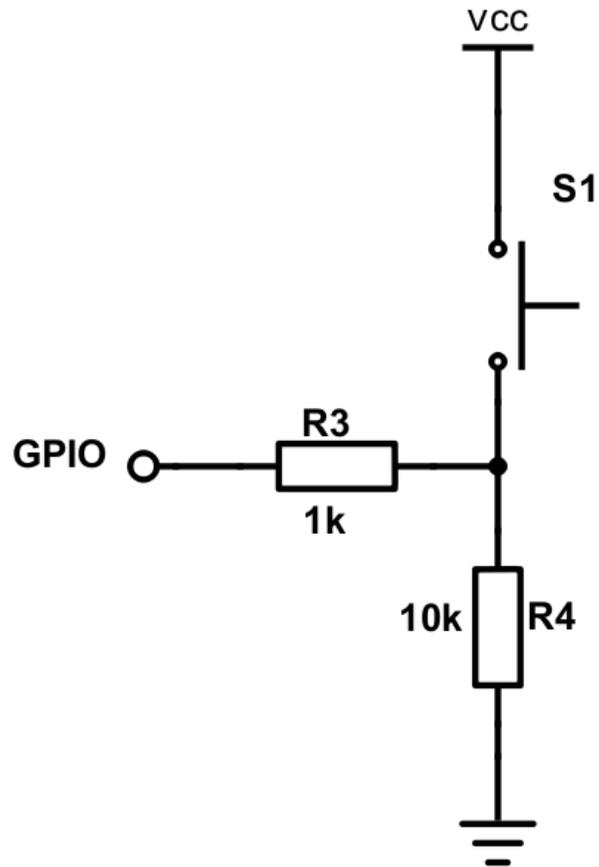
Figure 2. Button Switch Circuit Schematic
