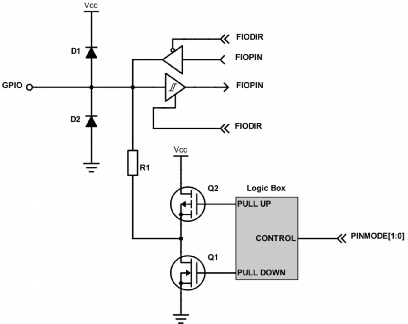
Figure 1. Internal Design of a GPIO
