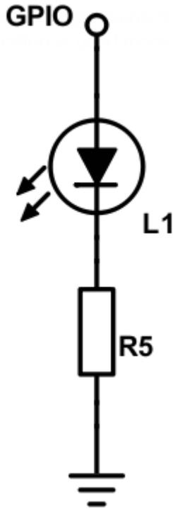
Figure 3. Active High LED circuit schematic
