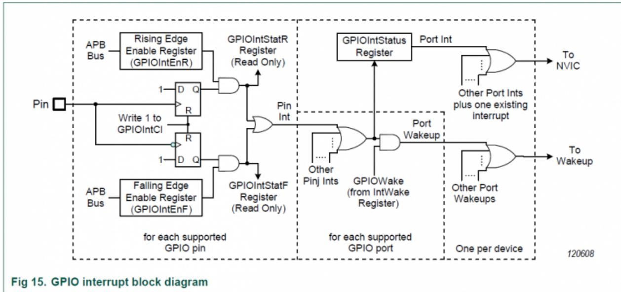
Fig 15. GPIO interrupt block diagram
