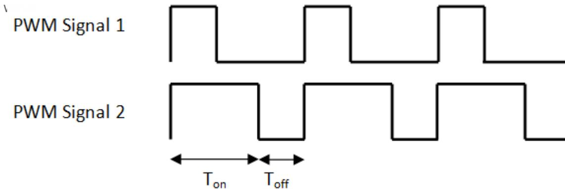
Figure 1. PWM Signal (credit: [www.bvsystems.be](http://www.bvsystems.be))
